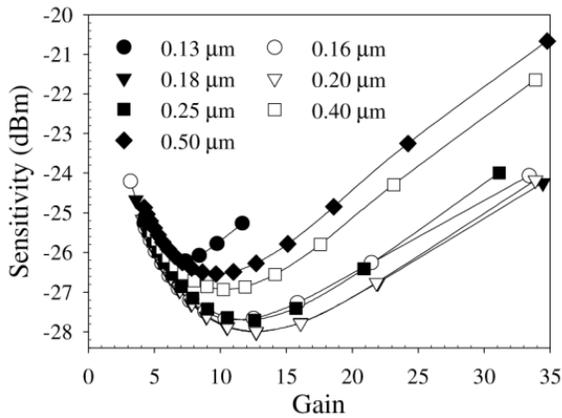
Fig. 1. Receiver sensitivity versus gain for the InP p-i-n APDs investigated for a  $10 \text{ Gb/s}$  transmission system.
