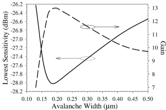
Fig. 2. Lowest sensitivity (solid line, left axis) and its corresponding optimal mean gain (dashed line, right axis) versus InP APD avalanche width for a  $10 \text{ Gb/s}$  transmission system.
