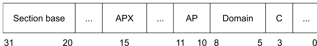
Figure 5.3: Simplified descriptor format for a 1MB section
