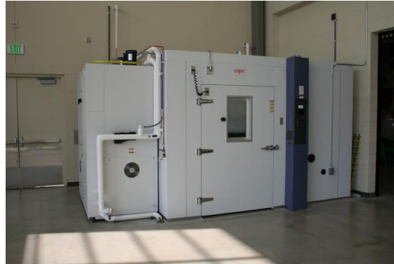
Figure 4. Walk-in Sized, ESPEC Temperature and Humidity-Controlled Room for Freeze/Thaw and Moisture Conditioning Testing
