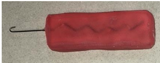
Figure 1. Testing apparatus: acrylic block enclosing .018-inch stainless steel wire with hook
