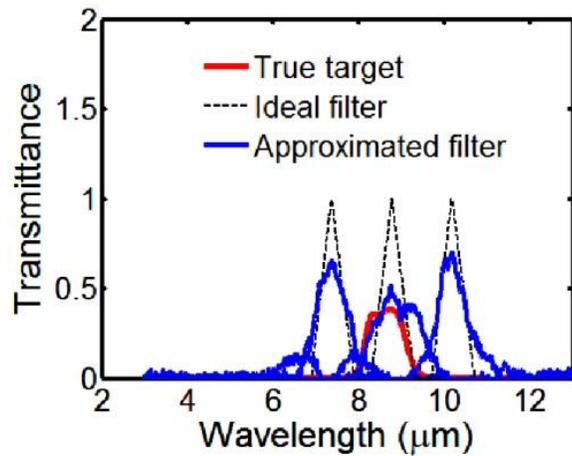
**Fig. 7** Three spectral filters,  $f_1(\lambda)$ ,  $f_2(\lambda)$  and  $f_3(\lambda)$  in the filter collection  $F_{MS}$  are used to sample the unknown target, whose transmittance is shown in red. For reference, the ideal triangular spectral filters are also shown in dashed line. Approximated filters in blue line were obtained by the UCSS algorithm using minimum four biases  $\{-3.0, -0.8, 1.0, 2.8 \text{ V}\}$  selected by the MBS algorithm.
