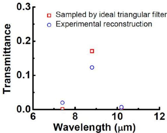
Fig. 8 Experimentally reconstructed transmittances (blue circle) at  $7.4 \mu\text{m}$ ,  $8.8 \mu\text{m}$  and  $10.2 \mu\text{m}$  extracted by the UCSS algorithm using minimum four biases  $-3.0, -0.8, 1.0, 2.8 \text{ V}$  selected by the MBS algorithm were obtained. Results are compared to the sampled transmittances by the ideal triangular spectral filters (red square) considered as the reference.
