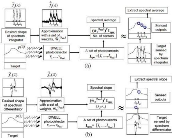
**Fig. 9** Applications of two linearly superpositioned filters (i.e., (a) the spectral integrator  $\tilde{f}_1(\lambda)$  and (b) the spectral differentiator  $\tilde{f}_2(\lambda)$ ) to the spectrometry problem of unknown filter target. Approximations  $\hat{f}_1(\lambda)$  and  $\hat{f}_2(\lambda)$  can extract the spectral average and slope of unknown target, respectively.
