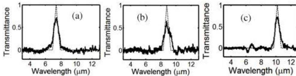
**Fig. 2** Example of three different narrowband tuning filter approximations centered at (a)  $7.4 \mu\text{m}$ , (b)  $8.8 \mu\text{m}$  and (c)  $10.2 \mu\text{m}$ , the algorithm requires 21 out of 30 biases. The biases used are  $\{-3.0, -2.8, -2.6, -2.2, -2.0, -1.8, -1.6, -1.4, -1.2, -0.8, -0.6, -0.4, -0.2, 0.2, 0.4, 0.6, 0.8, 1.4, 1.8, 2.4, 2.6\}$ .
