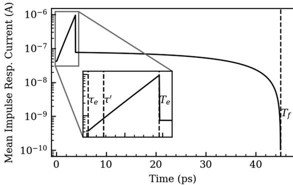
Fig. 2. Calculated mean impulse response for an InAs e-APD with  $w = 3.0 \mu\text{m}$  reverse biased at 18 V. The different stages of the mean impulse response function are indicated by the dashed lines in the figure.
