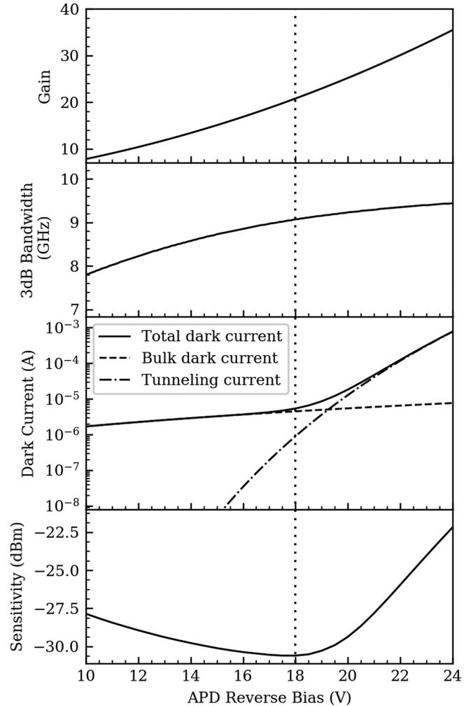
Fig. 3. Gain, 3 dB bandwidth, dark current, and sensitivity simulation data for a  $w = 3.0 \mu\text{m}$  InAs e-APD operated at 10 Gbit/s bit rate and  $1 \times 10^{-12}$  target BER. Its optimal operating voltage ( $-18 \text{ V}$ ) is indicated by the dotted line.
