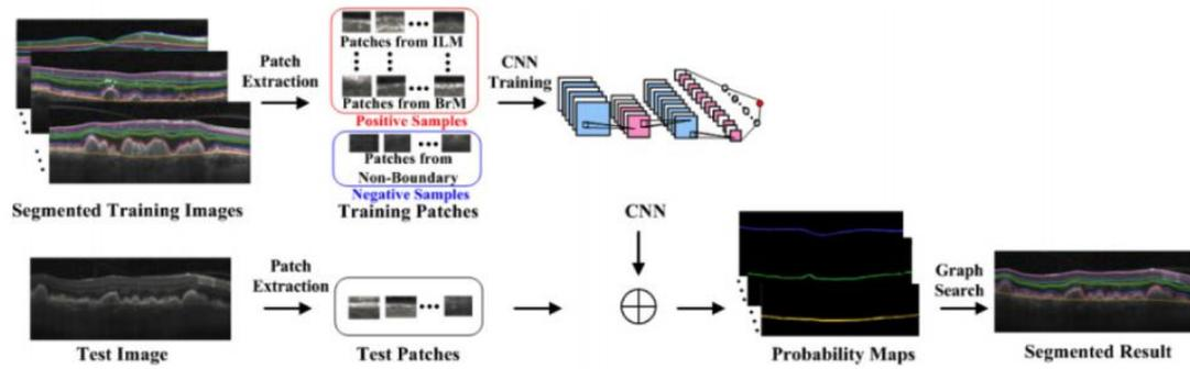
Figure 2.2 CNN-GS algorithm [39]
