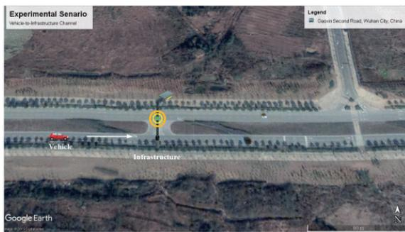
**Fig. 1.** Experimental scenario. (a) The transmitting antenna was placed on the roof of the test vehicle to minimize the multipath effect produced by the car. (b) The receiving antenna was placed on the road lamp post. Its height varies from 1 m to 9 m with an interval of 1 m.
