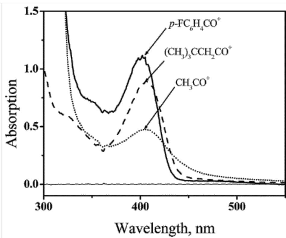
Figure 7 UV-vis absorption spectra observed at  $-70\text{ }^{\circ}\text{C}$  upon the addition of hexamethylbenzene to  $\text{CH}_2\text{Cl}_2$  solutions of acylium hexafluoroantimonates (as indicated).
