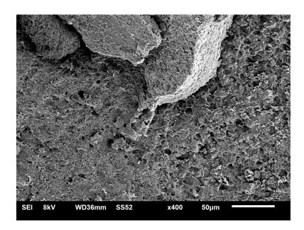
Figure 1c depicts no surface pre-treatment which showed rough rectangular patterns of irregularities Visio.link application and the site of fracture after the shear bond strength test was conducted.
