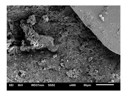
Figure 1e shows pre-treatment with a carbide rotary cutting instrument, Visio.link application and the site of fracture after the shear bond strength test was conducted.
