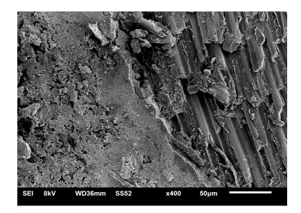
Figure 1d shows pre-treatment with Rocatec aluminum oxide particles and Silane application; Visio.link application and the site of fracture after the shear bond strength test was conducted.
