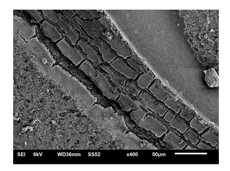
Figure 1b depicts surface pre-treatment with  $110 \ \mu m \ Al_2O_3$  showing circular porosities of the specimens Visio.link application and the site of fracture after the shear bond strength test was conducted.
