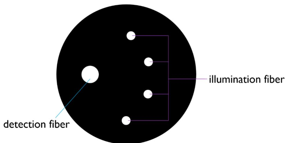
Figure 4.2: The geometry of the fiber-optic probe
