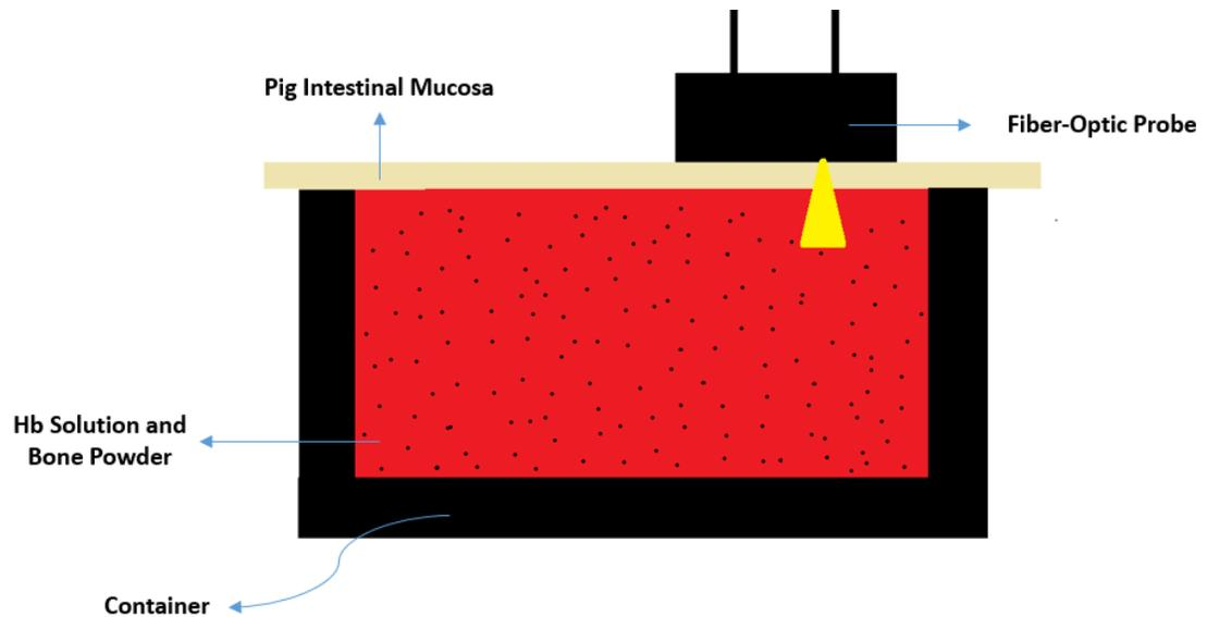
Figure 4.3: Experimental set-up to study the optical properties of a physical model simulating the mid-palatal suture after its response to expansion.
