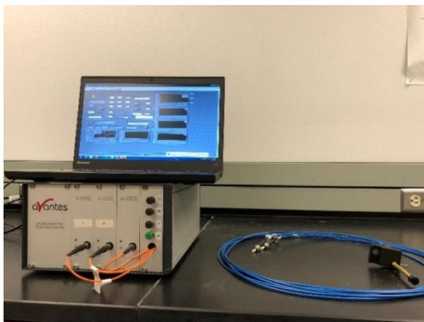
Figure 4.1: The fiber-optic DRS system with the fiber-optic probe
