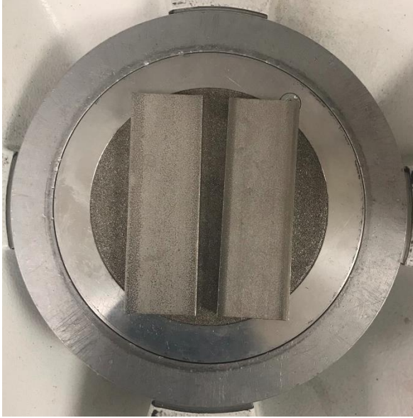
Figure 2. Rectangular stainless-steel blocks (1in x 2.5in x 0.25in) spaced apart on Biostar platform
