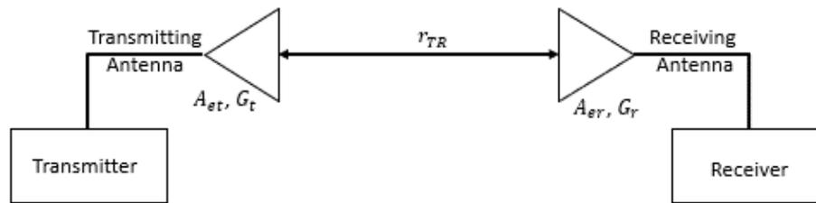
Figure 28. An example diagram of a wireless link telecommunication system between a transmitting and receiving antenna with area and gain of transmitter and receiver labeled. As well as length of the transmission signal between both apertures.
