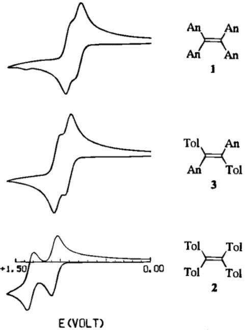
Figure 5 Cyclic voltammograms of 5 mM tetraarylethylenes 1, 2, and 3 (as indicated) in dichloromethane containing 0.2 M tetra-n-butylammonium hexafluorophosphate at a scan rate of v = 200 mV s<sup>-1</sup> (25 °C).
