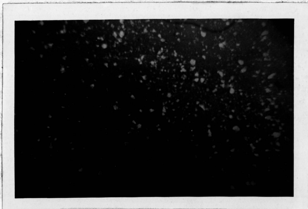
Figure 6. Microradiograph of iron powder taken with cobalt radiation. X60
