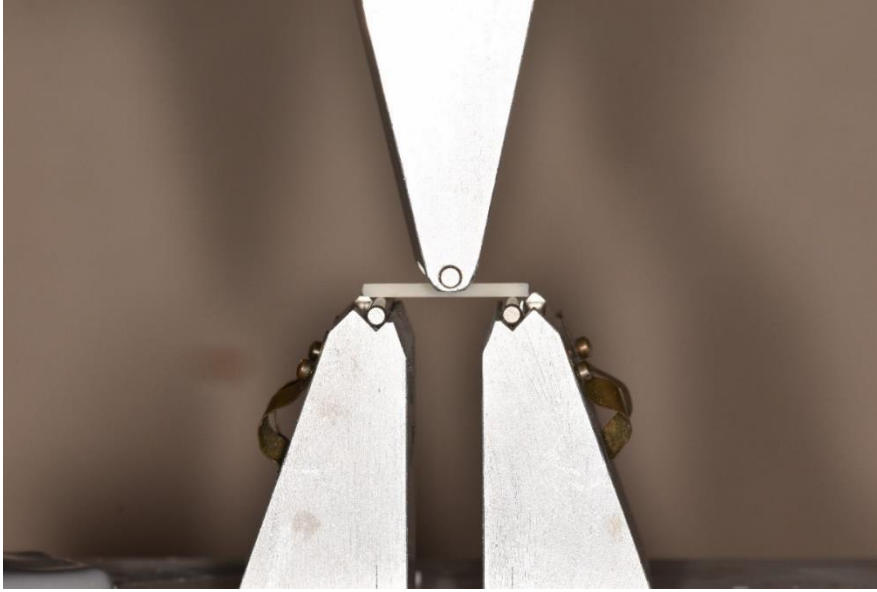
Figure 10: Chisel mounted on universal testing machine
