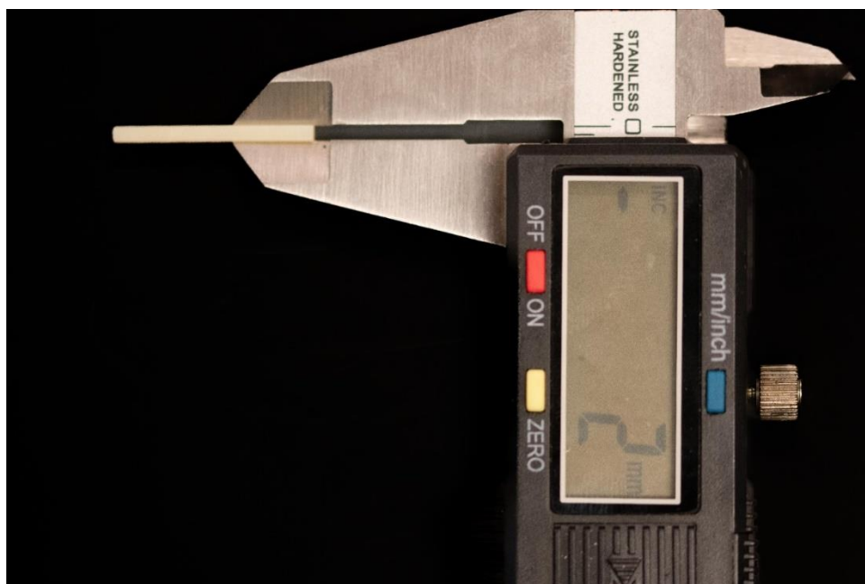
Figure 7: Mitutoyo caliper verifying dimensions.
