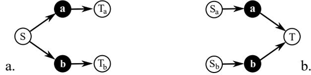
Figure 3.5: Bifurcation branch roadmap of a task path crossing a single coregular value. a) The roadmap of a task starting with 1 self-motion manifold and terminating with 2 self-motion manifolds. b) The roadmap of a task starting with 2 self-motion manifolds and terminating with 1 self-motion manifold.
