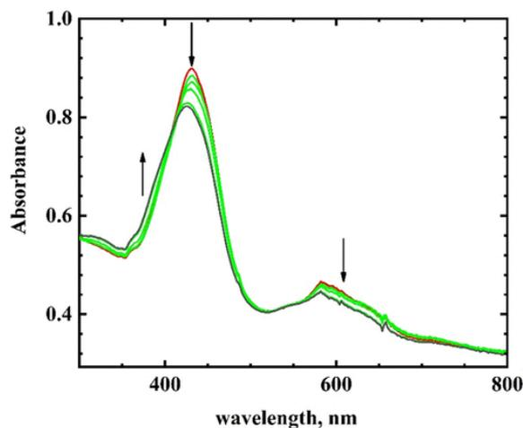
Figure 2. Visible spectroelectrochemistry for the second reduction of 0.3 mM  $\text{Fe}(\text{TpCF}_3\text{PC})(\text{NO})$  in THF. Initial spectrum:  $-1.706\text{ V}$  (black); intermediate spectra:  $-1.736\text{ V}$ ,  $-1.916\text{ V}$ ,  $-1.934\text{ V}^*$ , and  $-1.844\text{ V}^*$  (green); final spectrum:  $-1.754\text{ V}^*$  (red). \*Potential from reverse scan. Electrolyte:  $0.10\text{ M}$  TBAP.
