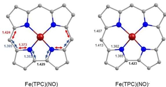
Figure 5. Bond length alternation in  $\text{Fe(TPC)(NO)}$  (left) as compared to  $\text{Fe(TPC)(NO)}^-$  (right). Bond lengths are in angstroms ( $\text{\AA}$ ).
