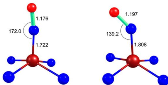
Figure 4. Central core of Fe(TPC)(NO) (left) and Fe(TPC)(NO)<sup>-</sup> (right). Distances are shown in angstroms (Å) and angles in degrees.
