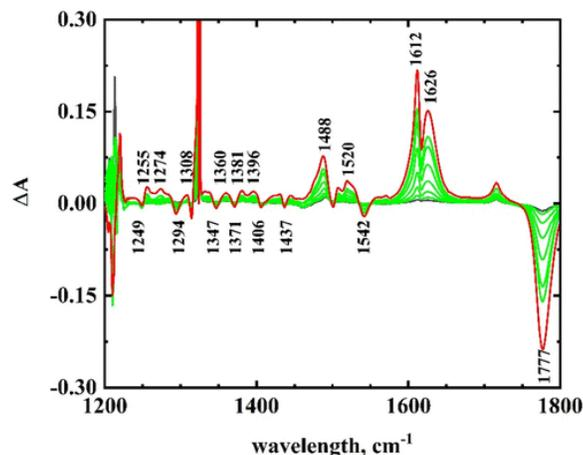
Figure 3. Infrared spectroelectrochemical difference spectra for the first reduction of  $4.5\text{ mM}$   $\text{Fe}(\text{TpCF}_3\text{PC})(\text{NO})$  in THF- $d_8$ . Initial spectrum (black); intermediate spectra (green); final spectrum (red). Electrolyte:  $0.10\text{ M}$  TBAP.
