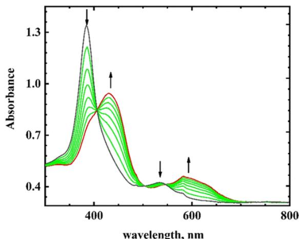
Figure 1. Visible spectroelectrochemistry of the first reduction of 0.3 mM Fe(TpCF<sub>3</sub>PC)(NO) in THF. Initial spectrum: -0.200 V (black); intermediate spectra: -0.551, -0.593, -0.620, -0.680, -0.730, -0.800 V (green); final spectrum: -0.701 V reverse scan (red). Electrolyte: 0.10 M TBAP.
