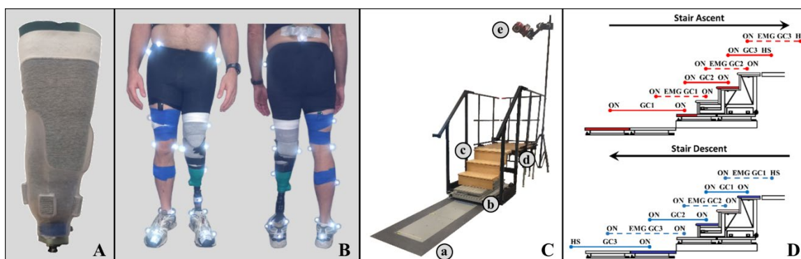
Figure 3.1. Electrode-socket integration and experimental walkway. (A) Individualized duplicate electrode-housing test socket and prosthetic shrinker used during amputee testing. (B) Modified Helen Hayes infrared lower limb marker set and EMG electrode placement on a transtibial amputee. (C) Experimental walkway including (a) embedded floor force plates, (b) stair force plates, (c) staircase, (d) landing platform, and (e) infrared motion cameras (APPENDIX D). (D) Schematic of step-over-step stair ambulation gait cycles (GC; red, stair ascent; blue, stair descent) used in the contralateral gait-cycle alignment. Gait cycles of the sound limb (lead limb) whose kinematics (ankle angle, shank velocities) and kinetics (ankle moment) were used as the target movement during training are shown as solid lines. Dashed lines denote consecutive gait cycles of the prosthetic limb (trail limb) whose residual EMG was aligned with the target kinematic/kinetic gait cycles.
