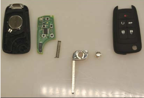
Figure 3. STRATTEC Key fob disassembly.
