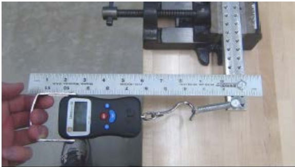
Figure 6. Spring rate measurement setup.
