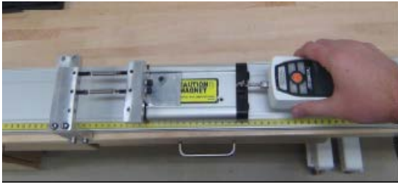
Figure 5. Determining stiffness of parallel springs with Pasco cart system and force gauge.
