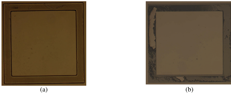
Figure 4. Optical images of pre-bonded post-test SU-8 structures (a) pre-bonded structure (b) post-test structure after separation with ~160-g tensile load.
