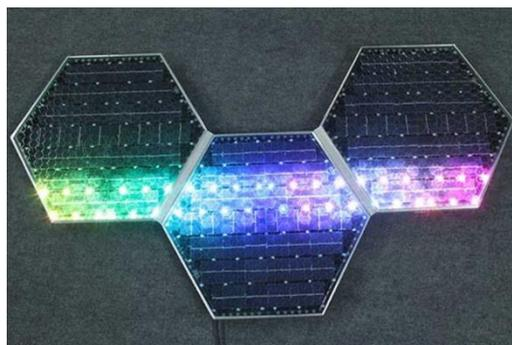
Figure 1. Solar Roadway, Inc. "SR3" Paver Panel (Brusaw, 2016)
