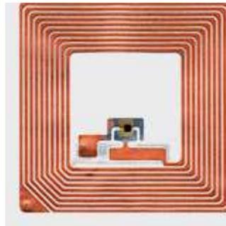
**Figure 1.1: An RFID tag (source: <http://www.barcode-solutions.com>)**
