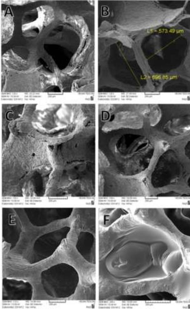
**Fig. 2.** SEM micrographs of  $\beta$ -TCP without coating (A–C) and with coating at concentration of 5% PLGA (D), 10% PLGA (E) and 20% PLGA (F).
